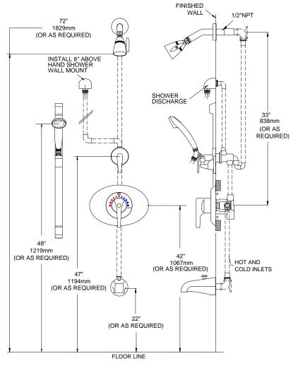
All Leonard Model 7600 Thermostatic Shower Valves have limitations. Please keep in mind that per the ASSE 1016-2011 Performance Standard, Harmonized along with ASME and CSA, it dictates inlet conditions of equal pressures, 45 PSI on both Hot and Cold Inlets, in addition to a Hot supply temperature range of 140 deg F-180 deg F. Significant deviations from those conditions stated above will alter performance expectations.
